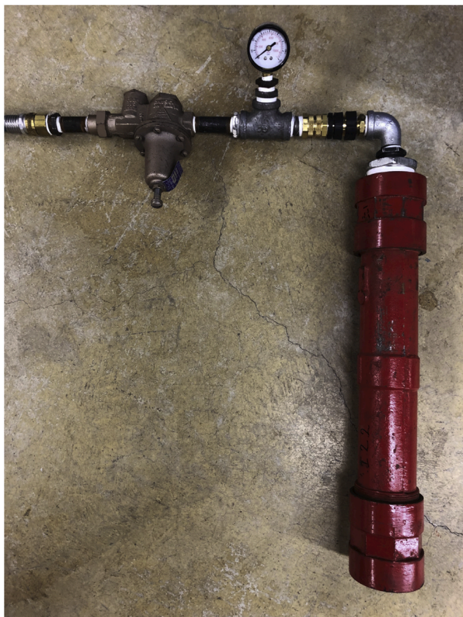
Fig. 10. Test setup for determining cup seal leak rate.
