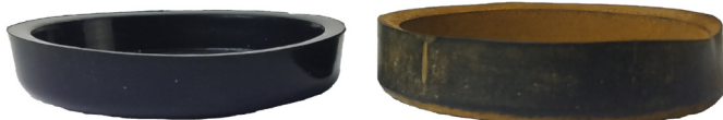
Fig. 8. New cup seal (left) and a used cup seal (right) for the India Mark II/III hand pump system.
