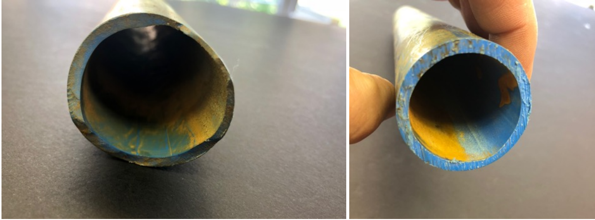
Figure A11.9. PVC pipe failure due to the pump rod being out of alignment.
