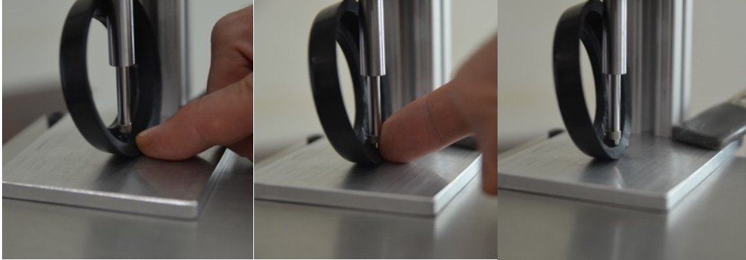
Figure A9.2. Measurement of the seal wall thickness.
