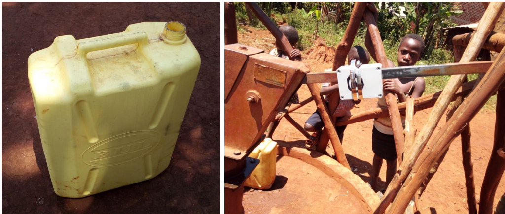
Figure A28.2. Jerry can used for test and placement of pump sensor.
