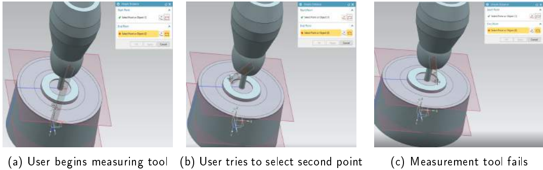
Figure 11: User cannot obtain dimensions. This was common in most envelope models where the layers were locked, making the geometry inaccessible
